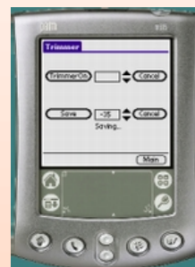
Active Test/ Active Setting: Use the active test monitor to test coils, injectors, tachometer, fuel pump relay, stepper motor, can purge solenoid, erase historic motor, can purge solenoid, erase historic errors and modify fuel trim.
